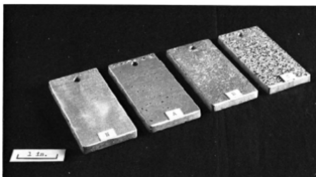
Fig.6 - ASSET Tested Exfoliation Resistant Specimens (N—No appreciable attack; A, B, C—Three Degrees of Pitting and Pit-Blistering)
