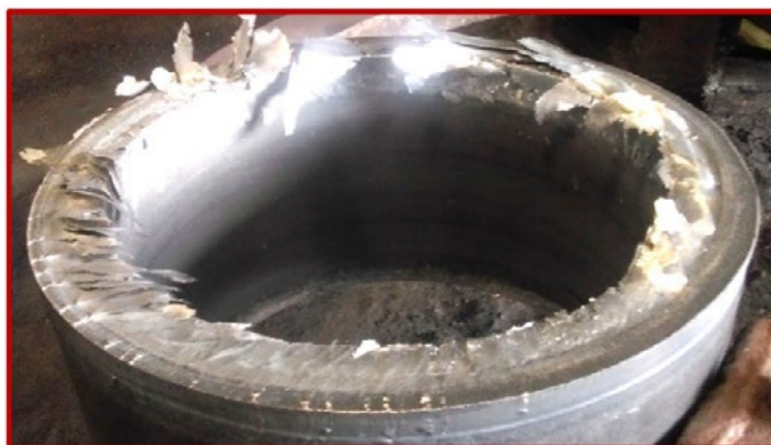
Fig.2 - Cold rolled ring (trial 3) showing heavy surface peel off and ring damage!
